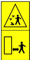
PIC. 2: Danger of being hit by flying fragments, cuttings, thrown objects, etc. Other people and animals - keep a safe distance from the machine.
