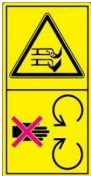
Pic. 3: : Do not reach into the working area of the rotary cylinder with your hands or step on your feet - risk of cuts.
